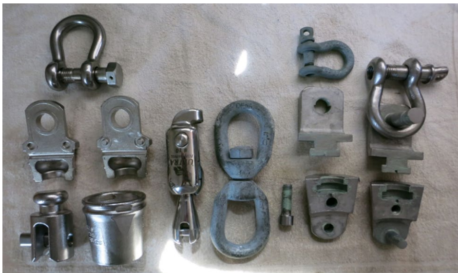
Anchor swivel types (left to right): disassembled Mantus, Ultra ball and socket Flip, Chinese galvanized 5/8" bail to bail, disassembled Kong. All have suitable ratings for 3/8" G4 chain.
